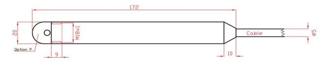
Level probe type B, BG: (preliminary size)
