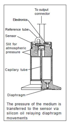
connected to ambient atmospheric pressure, via a tube, designed in order that air passes "cold surfaces" closest to the pressure connection of the transmitter. Any humidity in the air will condense on these surfaces. The condensate flows out and the remaining air in the tube stays dry. Additionally, the reference pressure connection is designed to prevent flushing water from entering.
