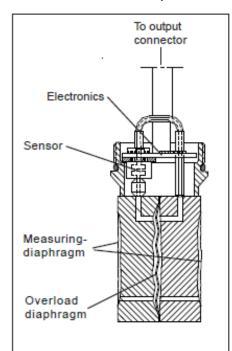
The pressure is transferred from the media to the sensor element via the separating diaphragms by means of silicon oil.
